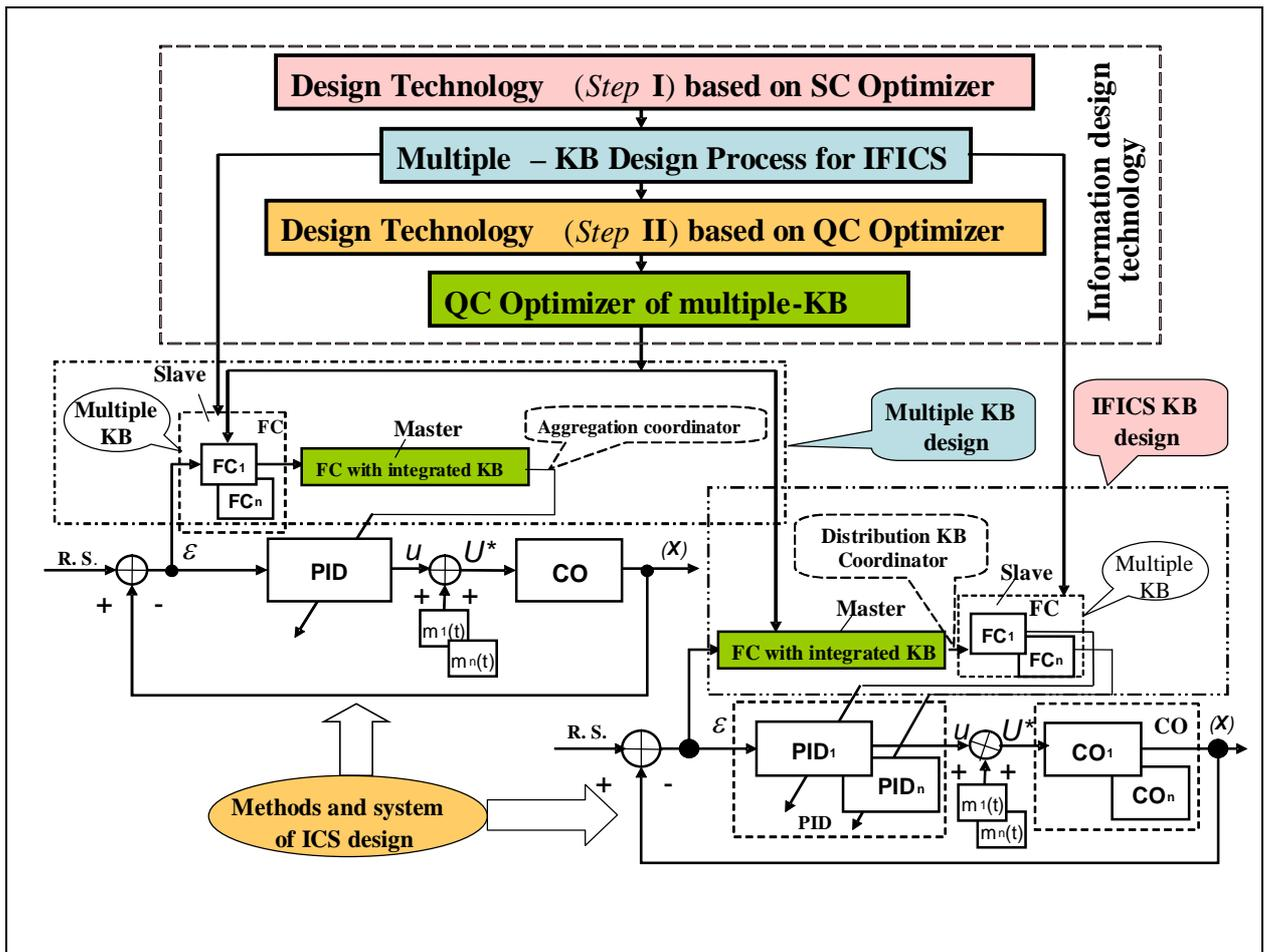
**Figure 1:** Structure of information design technology of IFICS
