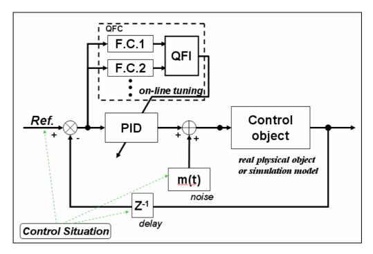
Figure 3: Main structure of intelligent self-organized control system
