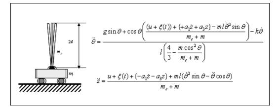
Figure 4: Cart-pole dynamic system: model and equations of motion
