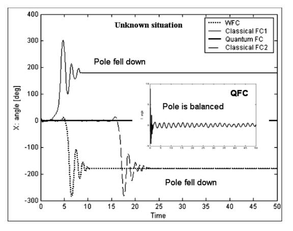
**Figure 6**: *Cart-Pole system - Unknown situation S4. Pole dynamic motion under different types of control*
