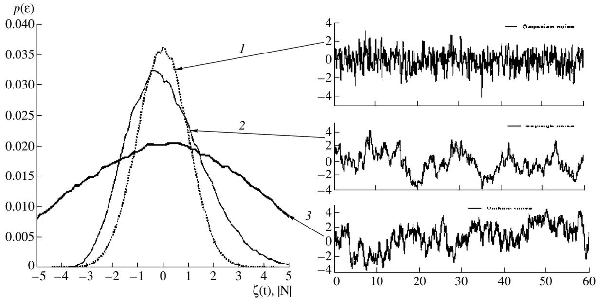
**Fig. 10.** The form of the density function of the probability distribution and the results of simulation of output stochastic processes from the corresponding forming filters: (1) Gaussian; (2) Rayleigh; (3) uniformly distributed.
