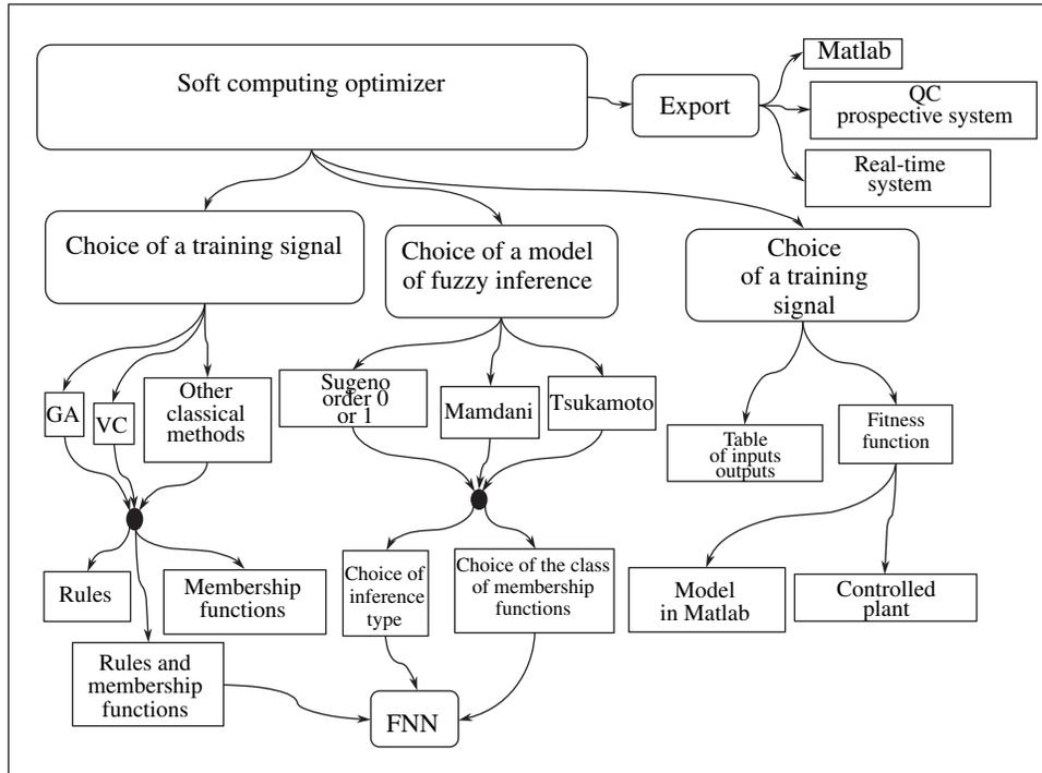
Fig. 26. The block diagram of the CSO.
