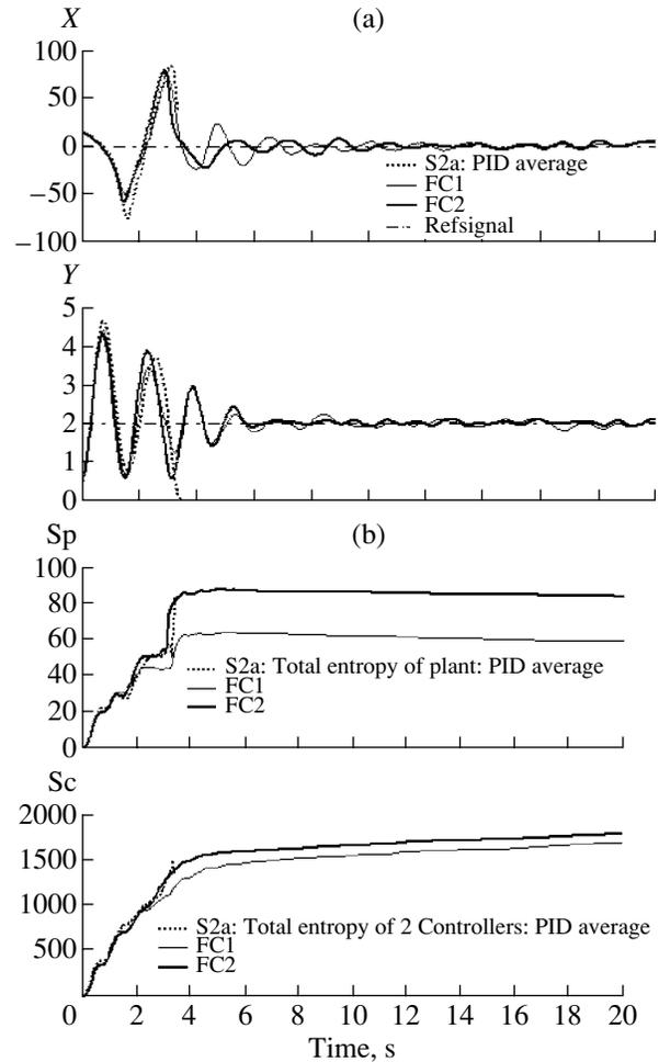
**Fig. 25.** The dynamic behavior of the CP in an unpredicted control situation (the description in the text): (a) loss of controllability of the PID controller; (b) entropy characteristics of the CP and controllers.
