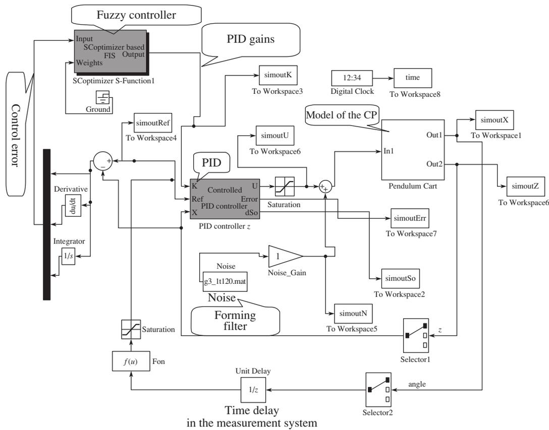
Fig. 9. A Matlab/Simulink Model of the control system.
